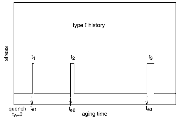
FIG. 1. Schematics of the protocol type I. The t_{ei} represent increasing aging times where t_{ei} \propto 2t_{e(i-1)} ( i=1, 2, \dots ). The t_i are the loading times and t_i/t_{ei}=0.1 .
